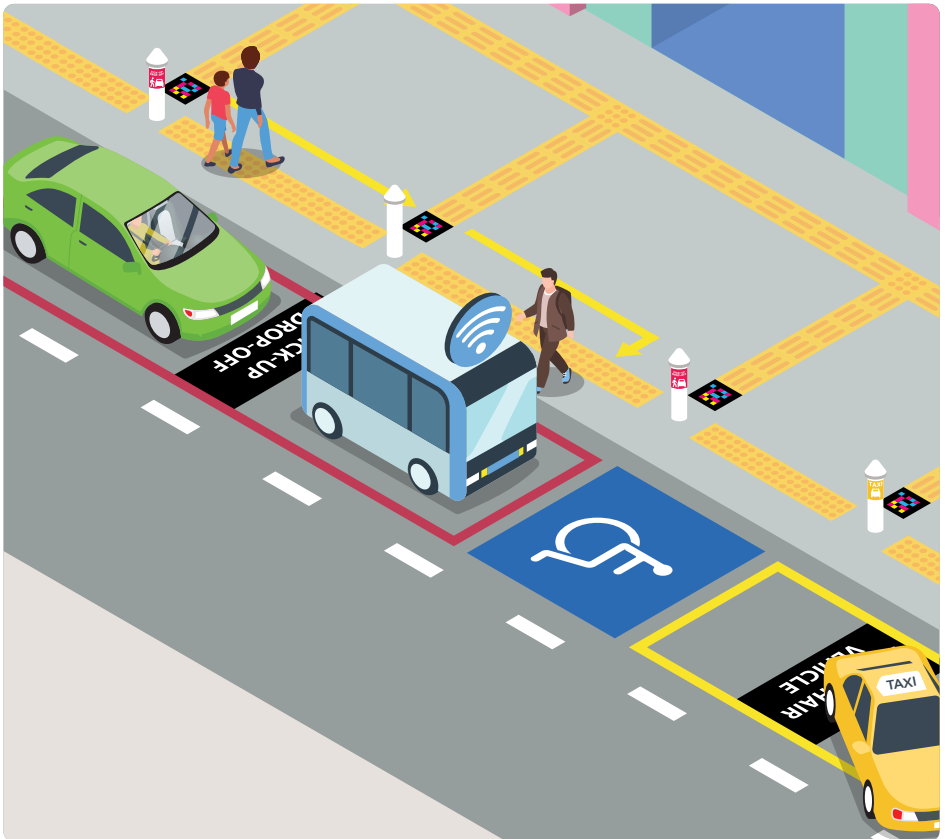
PUDO with differentiated berths for taxi and general pick-up and drop-off activities.
